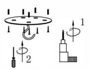
Screw on the plate with a suitable screw. Check that the plate is firmly anchored.
