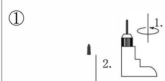
Determine the installation position, and then use the drill hole and buried plastic house lizard.
