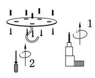
Screw on the plate with a suitable screw. Check that the plate is firmly anchored.
